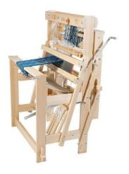
It is similar to a Laila but with 6 not 4 shafts. It is designed for weavers who do not have enough space for a very large loom, or who want an additional loom for sampling or experimental projects: a countermarch loom, it can be folded with the warp in place, and it occupies very little space when being stored or transported.
